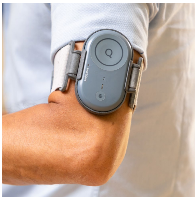
Fig. 1 The viQtor® wearable medical device (smartQare, Eindhoven, The Netherlands). The wearable sensor, attached to the upper arm, measures RR, HR, and SpO 2 using PPG signals. Additional features include skin temperature, activity index, and fall detection, which were not evaluated in this study
